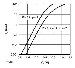
Fig. 5 - Typical Forward Current  $I_{\text{F}}$  vs. Forward Voltage  $V_{\text{F}}$
