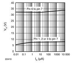
Fig. 6 - Typical Reverse Voltage  $V_{\mbox{\scriptsize R}}$  vs.Reverse Current  $I_{\mbox{\scriptsize R}}$
