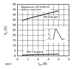
Fig. 8 - Typical Peak Clamping Voltage V<sub>C</sub> vs. Peak Pulse Current I<sub>PP</sub>
